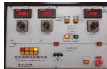
無載損及無載電流試驗 負載損及阻抗電壓試驗 Measurement of no-load loss and current Measurement of load loss and Short-circuit impedance test
