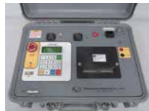
匝比及相位試驗 Measurement of voltage ratio and check of phase displacement
